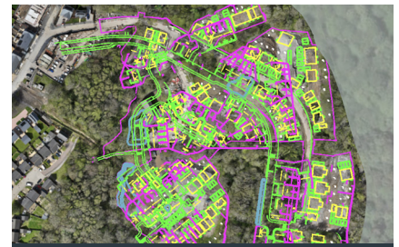
CAD Files overlaid on survey orthomosaic
